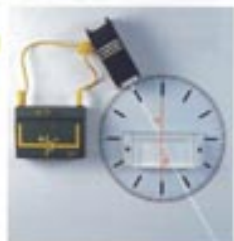
20 Angle of incidence and angle of refraction
