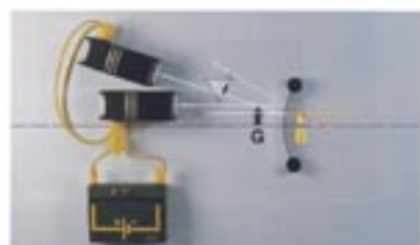
18 Path of rays when forming an image in a convex mirror
