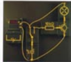
34 Discharging a capacitor
